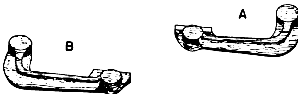
Figure 3-2. —Parted (split) pattern. 23. 67. 1
