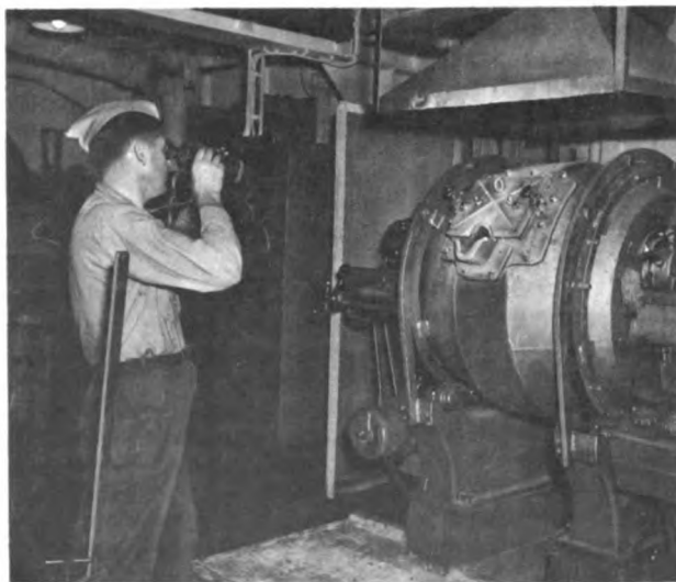
102.103 Figure 12-2. — Checking the temperature of the furnace charge with an optical pyrometer.
