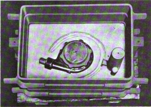
Figure 7-26. —Cope half of pattern and gating pieces set on the drag half.
