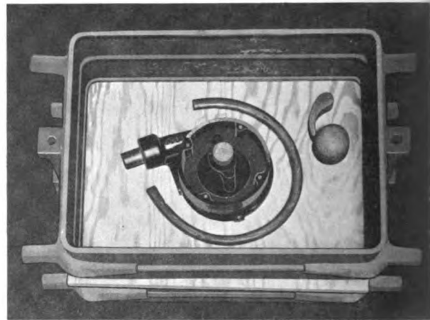
Figure 7-21. — Drag half of mold with pattern and gating system parts.
