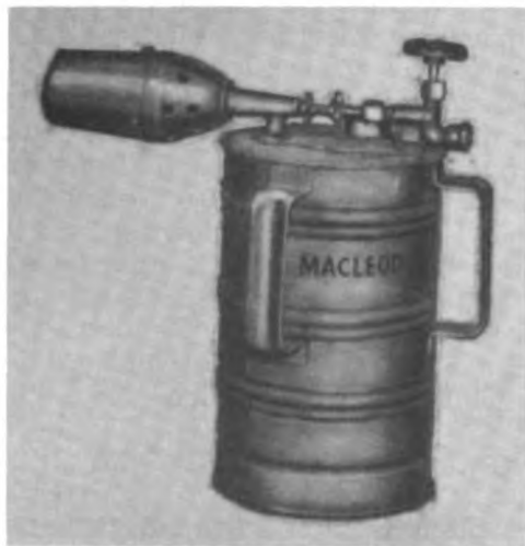
Figure 4-9. — Compressed air torch.
