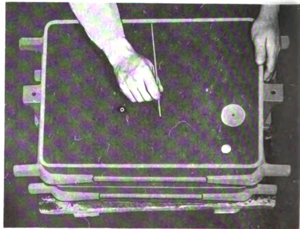
Figure 7-28. —Venting the cope.
