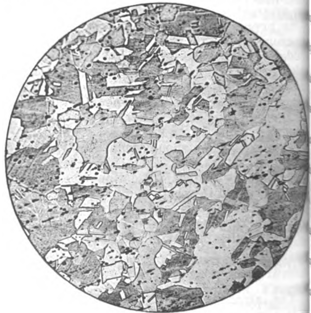
Figure 10-2. — Photomicrograph of pure copper
