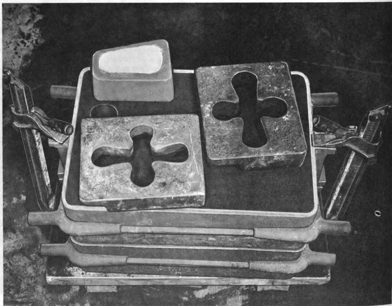
Figure 7-33. —The completed mold ready for pouring.
