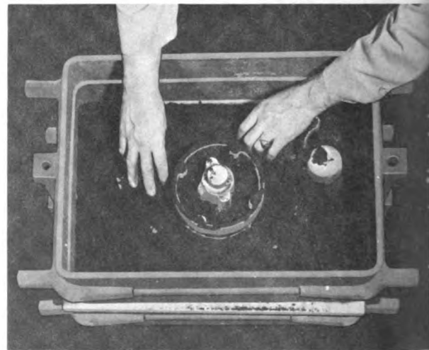
Figure 7-22.—Hand-packing riddled sand around the pattern.
